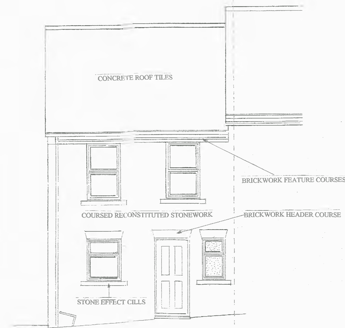
EXISTING FRONT ELEVATION
